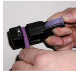
3. Clamp the cable firmly in the stripper. Using your thumb, tighten the cutting blades to strip the cable.
