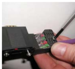
14. Rotate the cable clamp back towards the clear plastic connectors. Tighten down the cable clamp screw.
