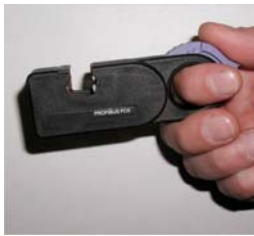
1. How to hold the insulation stripper in your right hand .
