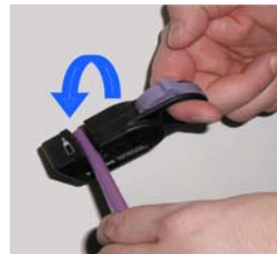
4. Rotate the stripper around the cable 4 times in the direction of the arrow (up over top of the cable.)
