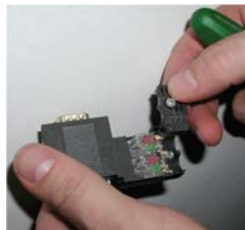
11. Rotate the cable clamp away from the cable connectors.
