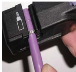
5. With the clamp still closed, pull the stripper off the cable. If the cut is not clean, replace the blade cassette.
