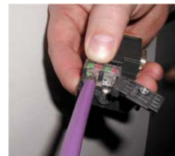
13. Insert the cable into the connector. The wires do not have to be stripped. These are insulation displacement connectors. Press down on the clear connector to make the connection.
