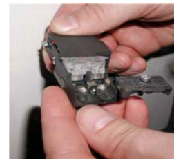
12. Lift up the clear plastic cable connectors. Be careful in not breaking the connectors.
