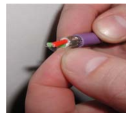
9. Pull the protective foil off the cores.
