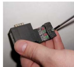
10. Loosen the cable clamp screw with a screwdriver.
