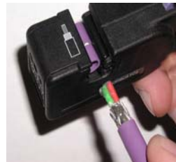
6. The removed insulation remains in the stripper. After releasing the clamp, the remnants can be removed.
