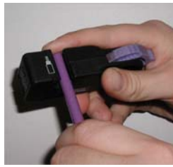
2. Match up the cable end with the end of the tool. Use the picture of the cable to point the cable in the proper direction.
